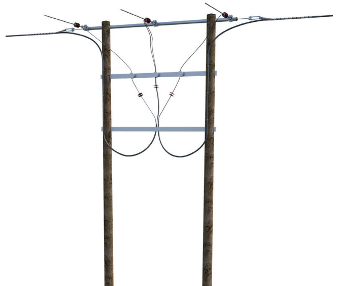
H-mast avgreining i topp blank line
