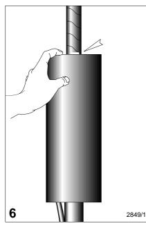
Slide the outer sleeve over the armour clamping rings. Position the top of the outer sleeve level with the mark on the cable.
