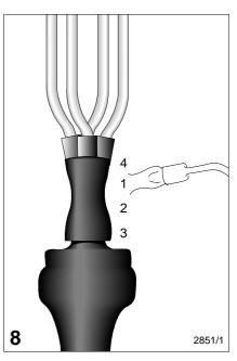
Remove the bedding and any filler at the end of the outer sleeve. Pass the breakout over the cores and pull it well down into the crutch.
