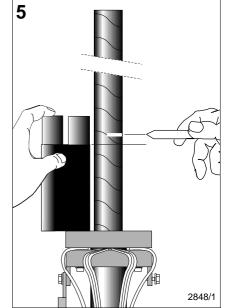
Screw the other clamping ring to the lugged clamping ring.
