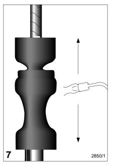
Shrink the outer sleeve into place starting at the centre. Shrink the lower end onto the armour wires and oversheath first, then the upper end.
