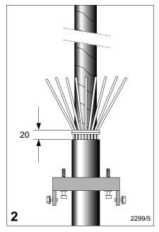
Disassemble the clamping rings. Slide one clamping ring lug-downwards over the cable. Bind the armour wires down with wire about 20 mm from the end of the oversheath.
