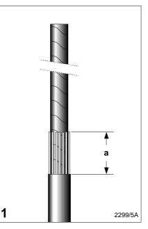
Trim the cable to the required length. Remove the oversheath. Remove the armour as shown in the
