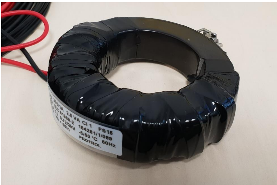
Figure 6: Split core current transformer of ring type with hose clamp for measuring current in a cable part.
