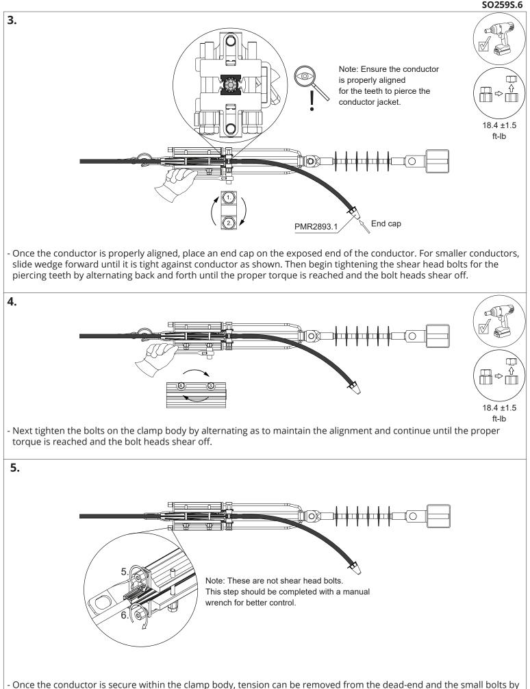
the bottom of the clamp can be tightened to remove slack.
