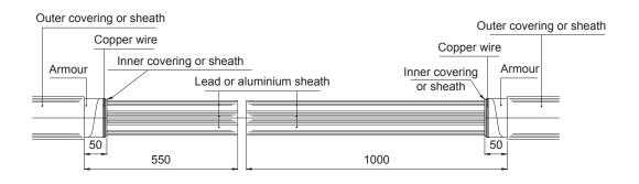
2. Cut and remove the outer covering or sheath for 550 mm on the short side of the joint and for 1000 mm on the long side of the joint. Cut and remove the possible armour up to 50 mm from the outer covering or sheath. Fix it with copper wire. Cut and remove the possible inner covering or sheath.
