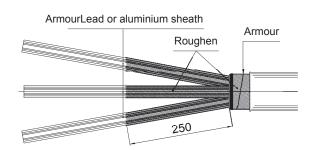
3. Clean the outer covering or sheath up to at least 1.5 m distance to avoid tube inner surfaces to become dirty. Spread the cores. Clean the possible armour and the lead or aluminium sheaths with a suitable solvent. Roughen the possible outer sheath for a distance of 100 mm and the possible armour for its length.
