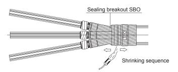
9. Push the sealing breakout SBO into the crutch as far as possible. Shrink the breakout starting from the middle.
