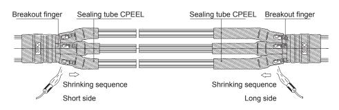
10. Place the longer sealing tubes on the longer cores and the shorter sealing tubes on the shorter cores. Push them on the breakout fingers up to about 20 mm from the crutch. Shrink the tubes one by one starting from the breakout end.
