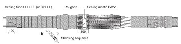
26. Slide the smaller CPEEPL (or CPEEL) sealing tube so that it overlaps 100 mm of the outer covering or sheath. Start to shrink the tube from middle and move towards the ends. The tube is properly shrunk when the adhesive starts to come out from the ends.
