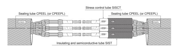
16. Slip the two sealing tubes CPEEPL (or CPEEL) one to each side of the cable, or both on the same side of the cable. The smaller one fits inside the bigger. Slip the insulating and semiconductive tubes SIST, the stress control tubes SISCT on the cores. Protect the tubes from dirt.
