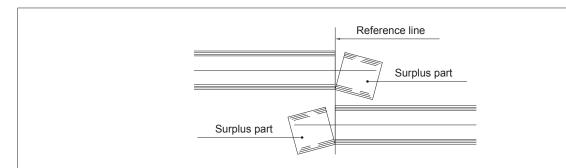
1. Overlap the cables for at least 300 mm. Cut the cables in the middle of the overlapping (reference line).
