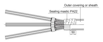
8. Wrap sealing mastic PA22 on the possible armour and continue to cover 50 mm of the outer covering or sheath. If there is no armour, just cover 50 mm of the outer covering or sheath.
