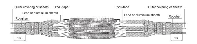
25. Cover the constant force springs with some layers of PVC tape. Cover also the open lead or aluminium sheath. Roughen 100 mm of the possible outer sheath on the both sides of the joint with grinding paper. Push the cores together.
