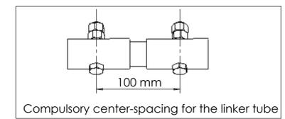
All tube-tube links are built using:
