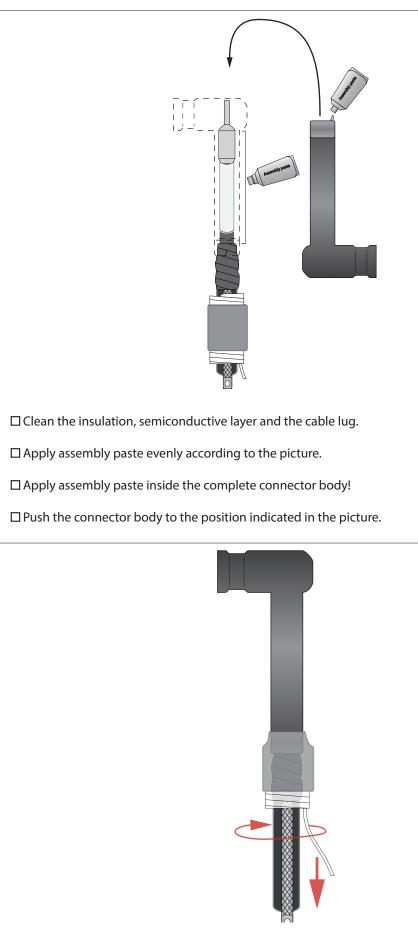
The spiral is removed by pulling it while turning it counter-clockwise.
