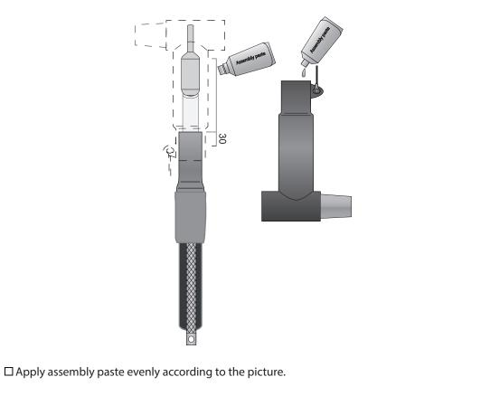
□ Push the connector body to the position indicated in the picture.
