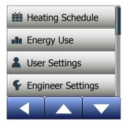
The main menu consists of four options which can be used to configure your thermostat.
