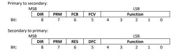
The RES and DFC bits relate to control fields for secondary stations to primary stations. They are replaced by the FCB and FCV bits for exchanges from the primary station to the secondary station. See standard IEC 870-5-2.
