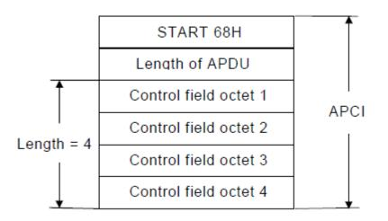
The specified data bytes are represented in hexadecimal notation as defined by IEC 870-5-1. The fixed frame length is 6 bytes.
