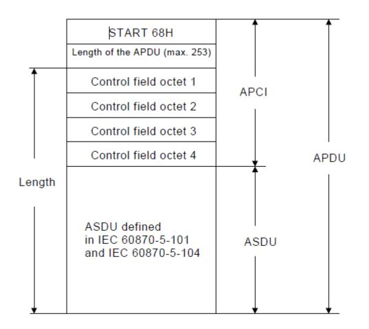
The specified data bytes are represented in hexadecimal notation as defined by IEC 870-5-1.
