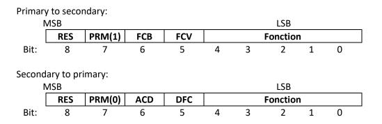
The ACD and DFC bits relate to the control fields for secondary stations (instrumentation & control cabinet) to primary stations (SCADA). They are replaced by the FCB and FCV bits for exchanges from the primary station (SCADA) to the secondary station (instrumentation & control cabinet). See standard IEC 870-5-2.
